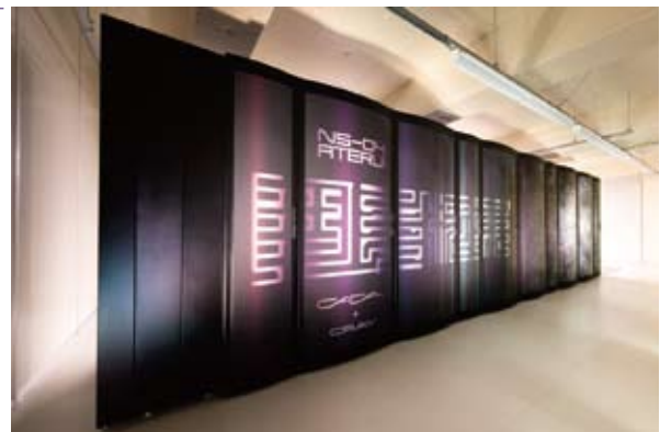
The fastest supercomputer for astronomy, Cray XC30 "ATERUI." Its peak performance is approximately 1 Pflops (1 quadrillion calculations per second).
