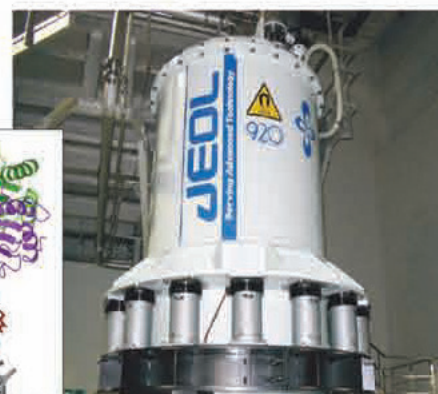
The molecular structure of protein is unveiled by measurements using an ultra-high magnetic field NMR apparatus.
