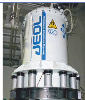
The molecular structure of protein is unveiled by measurements using an ultra-high magnetic field NMR apparatus.
