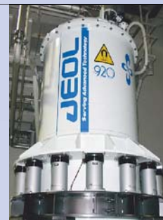
The molecular structure of a glycoprotein is unveiled by measurements using an ultra-high magnetic field NMR apparatus.
