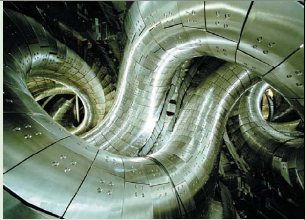
The LHD vacuum vessel
