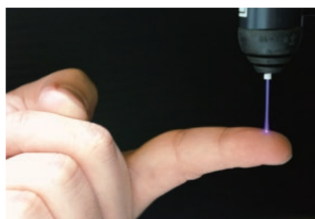
Low-temperature atmospheric pressure helium plasma jet that can be directly irradiated to the living body.
